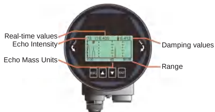
Figure 6-2 Schematic diagram of the echo curve interface
