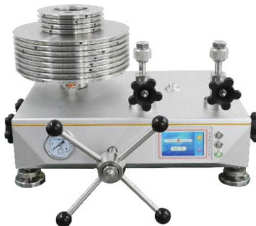
QY pneumatic dead weight tester
