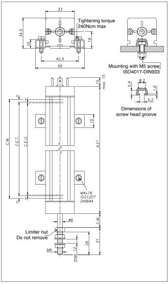
**Important**: all the data reported in the catalogue linearity, lifetime, temperature coefficient are valid for a sensor utilization as a ratiometric device with a max current across the cursor  $lc \le 0.1 mA$
